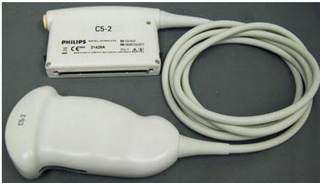
Figure:10. Philips C5-2 curvilinear ultrasound probe.
